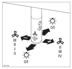
The joystick controls the fan power and overhead lighting.
